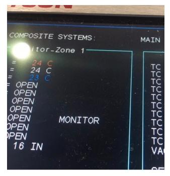
The image below represents the variations in temperature collected by censors in the three locations on the mild steel panel a minute after heat was applied.
