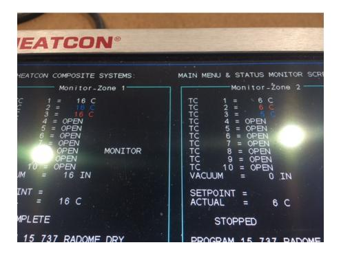
The Aluminium panel when subjected to lower temperatures showed no noticeable temperature variation in any of the three censor locations.
