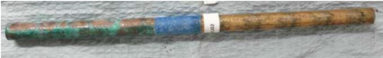
Fig 1: LG2 Bronze sample - Untreated and Treated after 400 hours neutral salt spray exposure.
