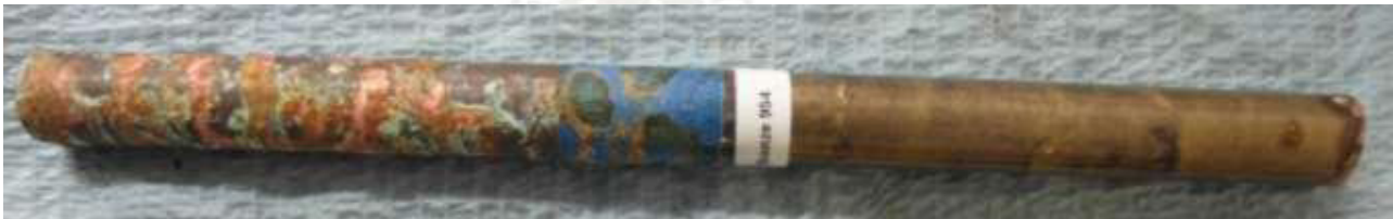
Fig 2: 954 Bronze sample - Untreated and Treated after 400 hours neutral salt spray exposure.
