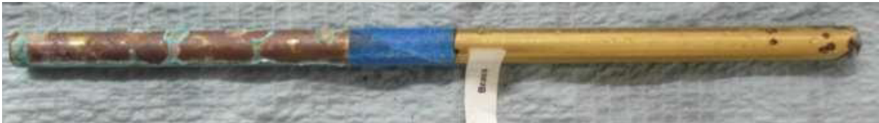
Fig 3: Brass sample - Untreated and Treated after 400 hours neutral salt spray exposure.
