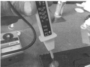
The censor probe was placed on the surface of the same steel plate where the Action Clear Coat had been applied. The Voltage tester did not illuminate indicating there was no current on that surface.
