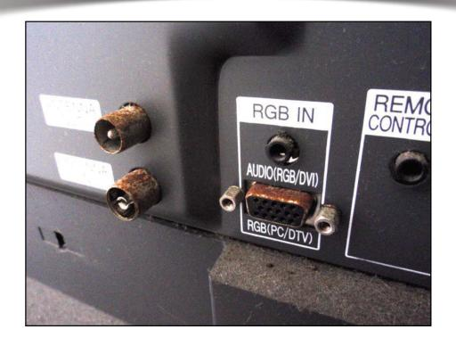
The terminals of this television have corrosion due to it's proximity to the sliding door. Internally it will have similar issues. New age T.V's generate more heat and have many ventilation holes in the rear which provides an easy access point for salt and dust. Wipe down these areas and treat with a electrical corrosion inhibitor.
