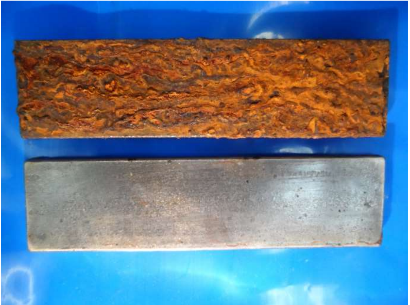
Mild Steel Control Top Mild Steel Action Clear Treated Bottom Samples after 291 Hours NSS testing
