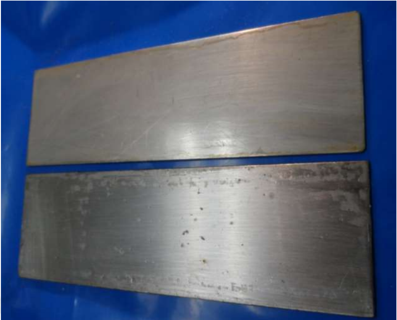
304 Stainless Steel Control Top 304 Stainless Steel Action Clear Treated Bottom Samples after 291 Hours NSS testing
