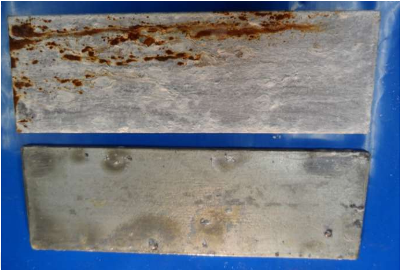
Galvanised Steel Control Top Galvanised Action Clear Treated Bottom Samples after 291 Hours NSS testing
