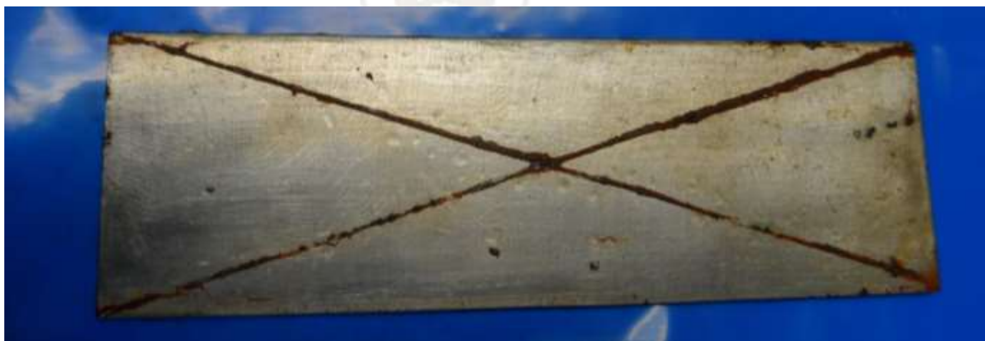
Mild Steel Control Cross Etched Sample after 291 hours NSS testing
