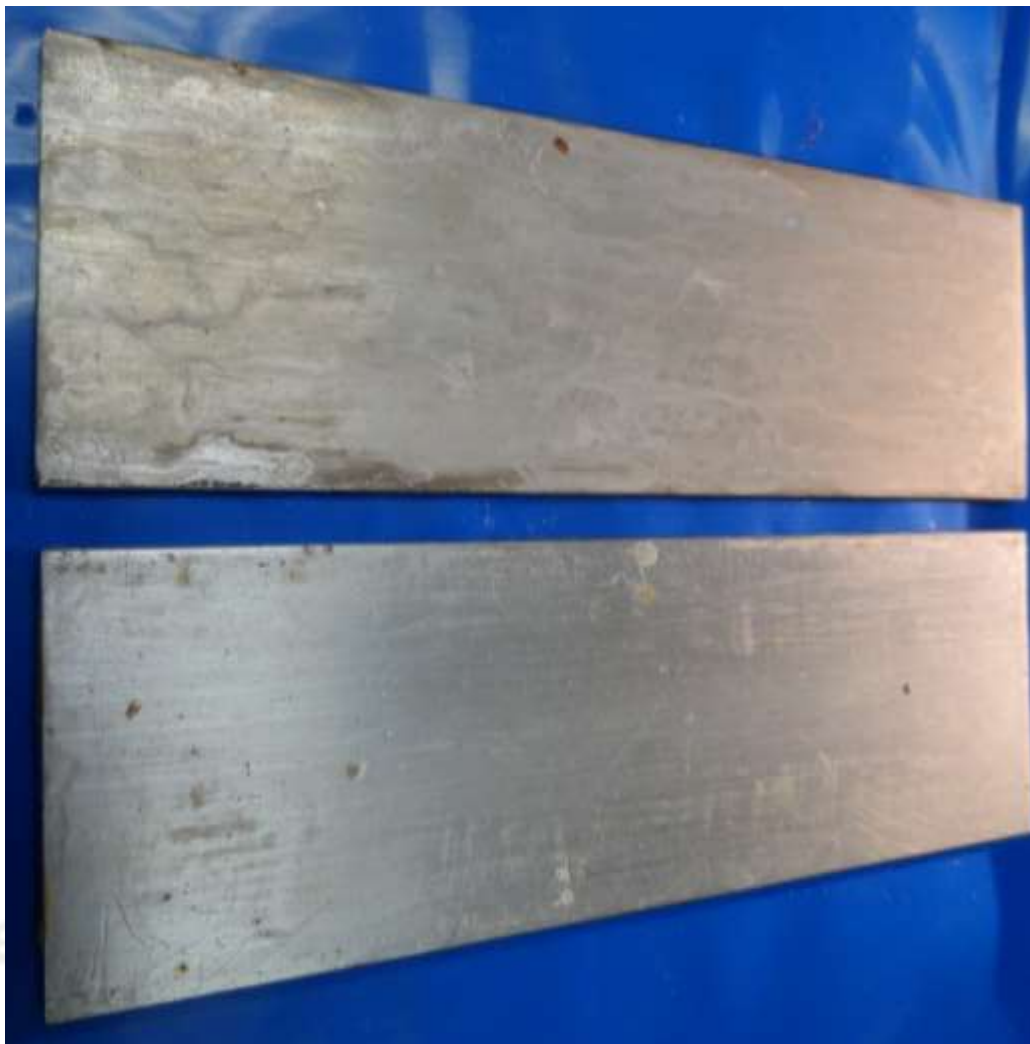
Aluminium Control Top Aluminium Action Clear Treated Bottom Samples after 291 Hours NSS testing
